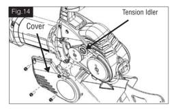
If excessive slipping has occurred, the pulleys can become worn. A worn pulley is evidenced by the groove having lost its well defined "V" shape, resulting in a rounded or flattened groove. To replace either pulley, contact your ARBORTECH authorised service centre.
