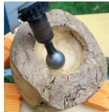
▲ The 30mm-diameter blade rotates at 12,000 rpm, gently peeling away the stock to create a cove.
