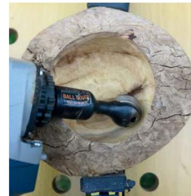
▲ The ball gouge allows you to nibble away at an edge, producing undercut edges with ease.
