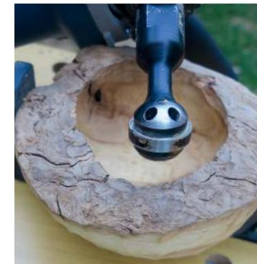
▲ The self-sharpening disc hones itself after each pass. The active edge is between the "dots".
