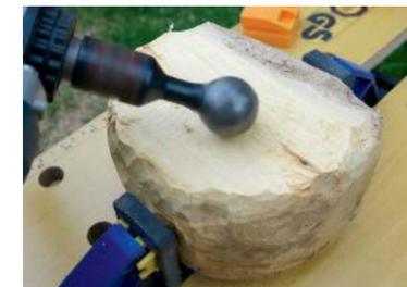
▲ A smooth sweeping motion is used to create flat surfaces. A steady hand is the key.
