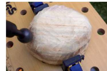
▲ The ball gouge can be used just like a traditional gouge and used to produce spiral scallops.
